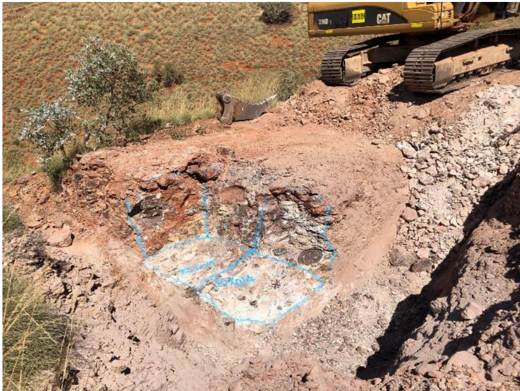
Figure 7-11. Tightly packed armored lag type ferruginous conglomerate with quartz boulders (M1 - Edwards Lease).
