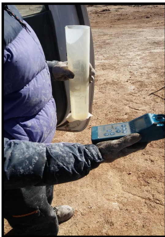
Photo 3: In situ measurement of physicochemical parameters of brine.
