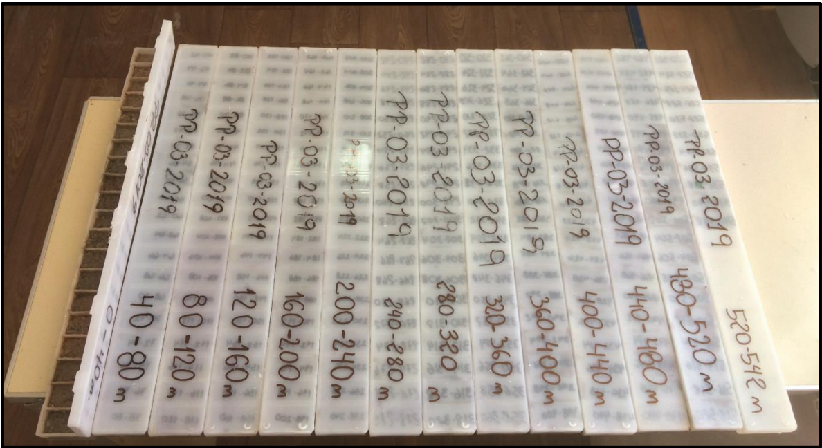
Photo 5: Samples described (0-542 m depth), labelled and stored sequentially in cutting boxes.
