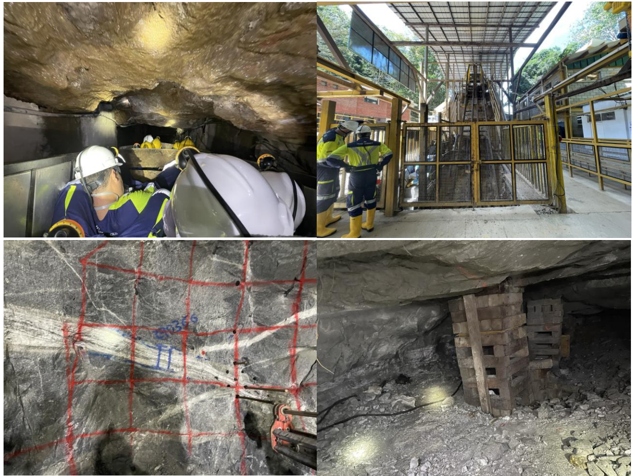
Figure 5: (clockwise from top left) Descending into El Silencio via a skip in an inclined shaft, Top of an inclined shaft at surface at El Silencio, Pillar recovery at El Silencio ~800m below surface, 1040 vein present in mine face on level 30
