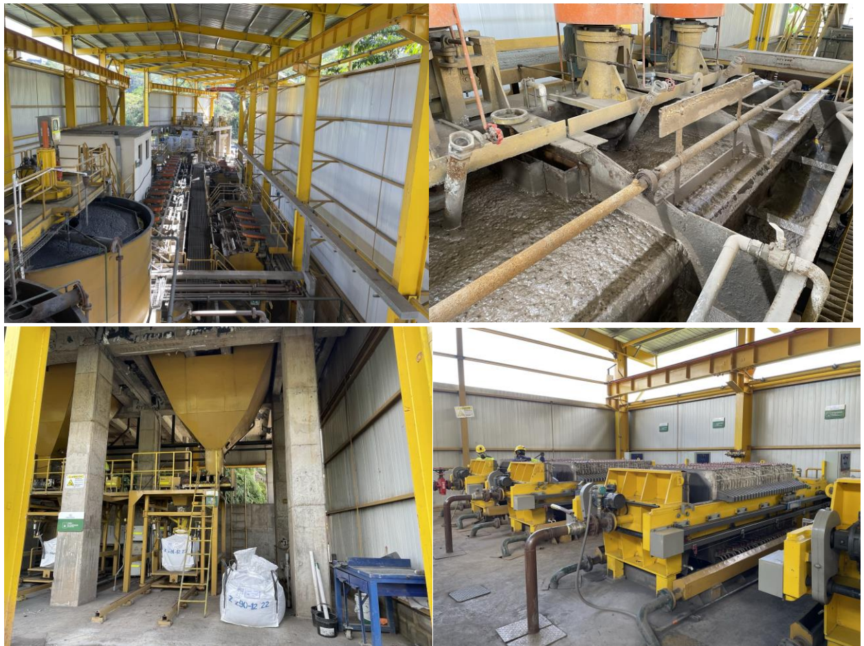
Figure 8: (clockwise from top left) New polymetallic plant with two lines (Zn and Pb), Cleaner Zn cells, Filter presses, One of two packing machines
