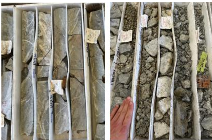
Fig 5 Site visit core photos – Left: Competent cut core from Napoleon, showing excellent +80% RQD conditions. Right: Poor cut core from Napoleon with crushed rock and minor gouge, estimated to be <20% RQD.
