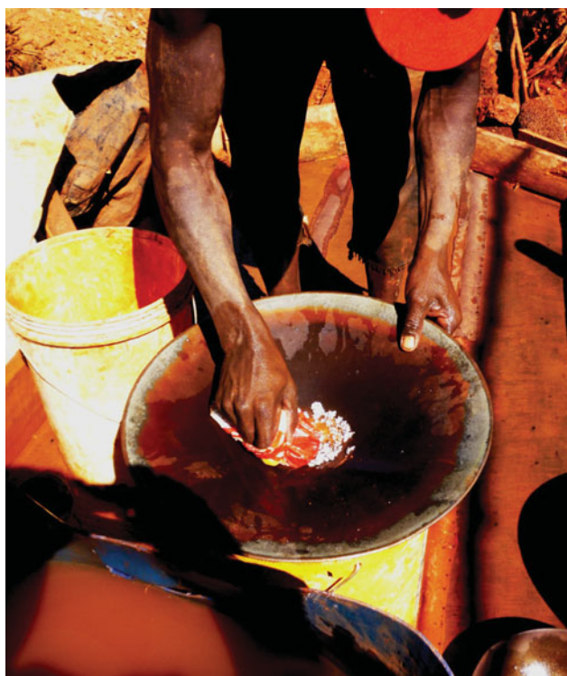
Fig. 8. Mercury recovery of gold in batea (gold pan) (photo: R. Finkie).
