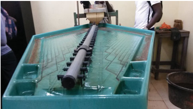
Fig. 10. Shaking table at Maripaston gravity concentration plant (photo: R. Finkie).
