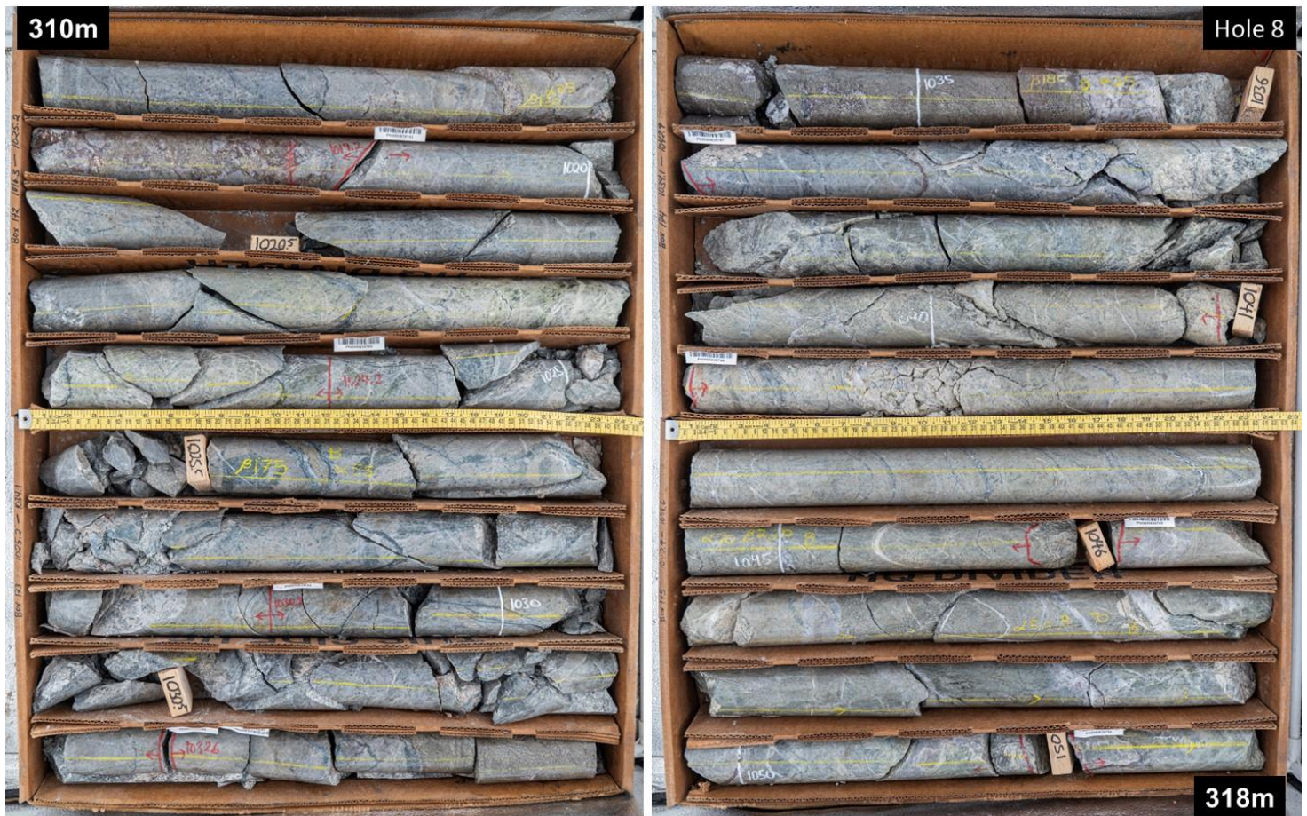
Fig 5 Core photos, hole 8 (310m to 318m downhole) – Showing a sub-interval of 32m at 0.67%Cu, 2g/tAg, 0.01%Mo (0.70%CuEq) within 437.5m at 0.32%Cu, 0.01%Mo (0.35%CuEq) within strong phyllic alteration bearing abundant pyrite-chalcopryrite+/-bornite sulphide mineralization in quartz veins with sericite selvages. We highlight the high density of what look like sulphide-rich “D” veins and qtz-sulphide “B” veins, suggesting hole 8 was drilled in a distal part of a very robust mineralizing system.
