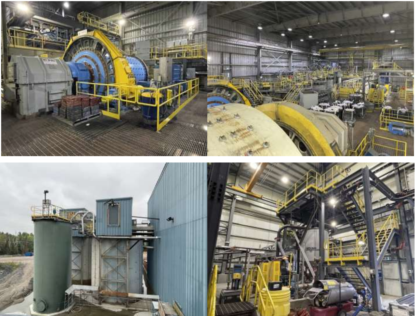
Figure 40: (clockwise from top left): new ball mill at Madsen Mill that could be replaced with a larger one in expansion scenario, interior of Madsen Mill, new paste plant, tanks with room for additional tanks required in expansion scenario
