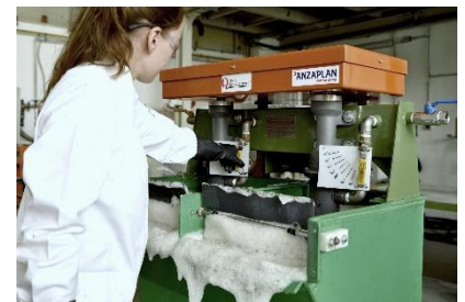
Figure 4: ANZAPLAN technician conducting flotation experiment
