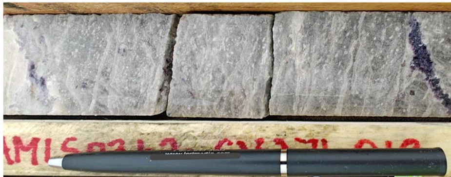
Figure 35 - Pollucite Mineralisation in High-Grade Caesium Drill Intercept
