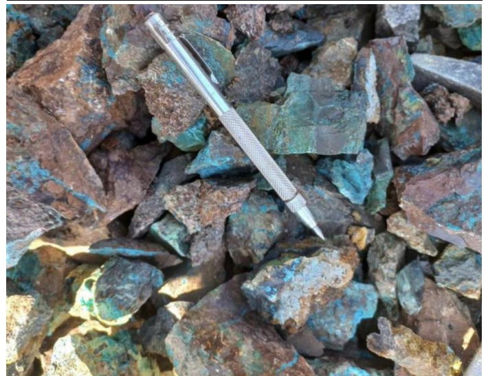
Figure 28: High-grade from Flor de Espino vein – Upper Level (oxides)
